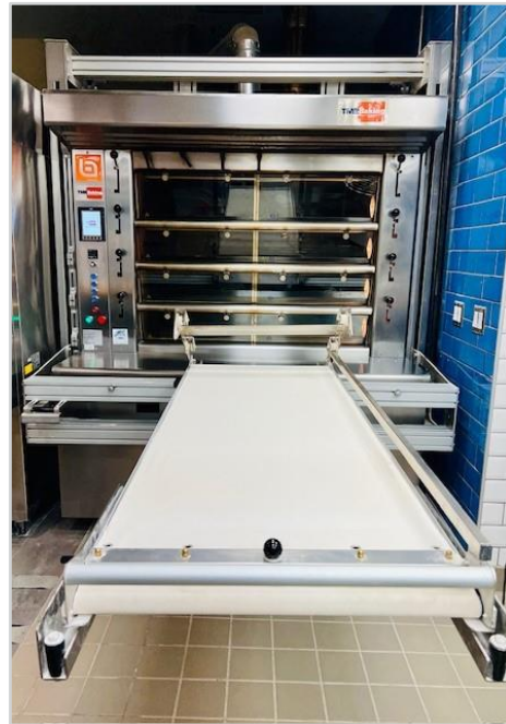
Shown: Zoom 1212 with TMB Touchscreen Control & Integrated Loader (Otto's Bread Company, Salinas, CA)
