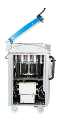
Daub Robocut models are available with both round and square dough bowls. A round (47 x 12 cm) bowl for optimal weight accuracy. A square (43 x 43.5 x 12 cm) bowl for easy to handle dough portions. Both versions are available in various dough weight ranges.
