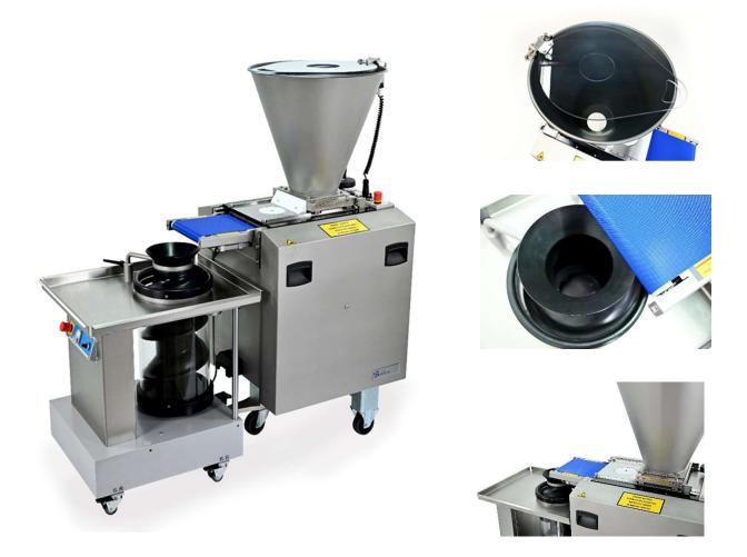
Daub's SLIM Globe Divider Rounder is specially designed for a wide range of food-processing environments with high demands on dough quality and weight consistency.
