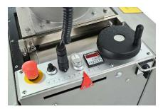
The SLIM Globe is designed for daily use. The machine is equipped with electronic speed control and piece counter.
