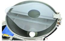
Stainless steel hopper for 50 kg or 90 kg of dough. With teflon coated interior no dough is left behind in the hopper.
