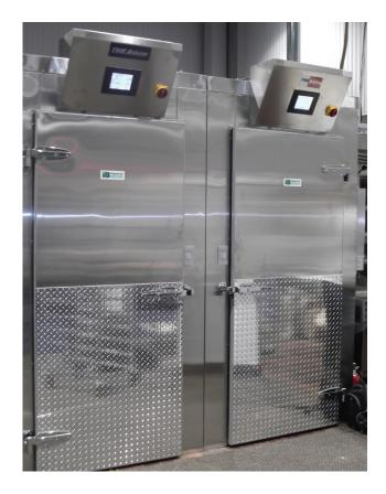
**Dough 'Conditioning'–** TMB Baking technicians specify the right quantity of our custom design air diffuser equipment (stainless steel reverse evaporators) inside the box to 'condition' the air to meet your objectives.
