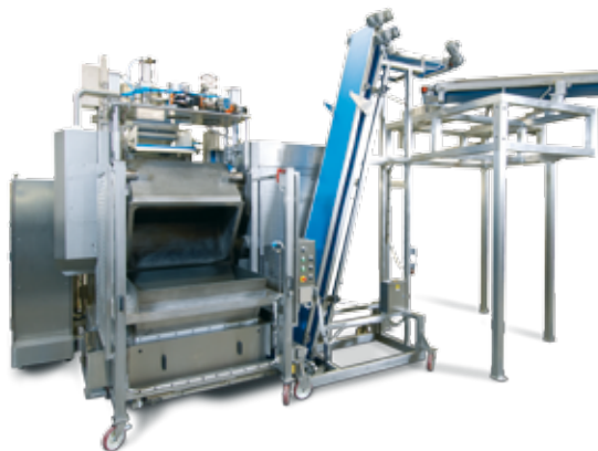
Verymix III horizontal kneading under vacuum
