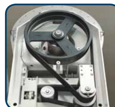
Mechanical reduction with pulleys and belts
