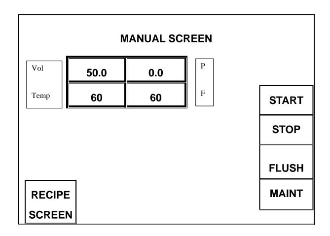
To set up water or temperature, touch the volume or temperature button. Screen will change to:
