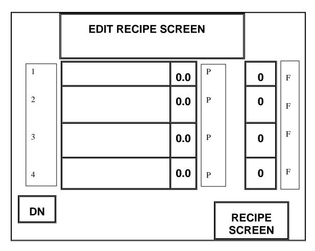
To prevent accidental changes in the recipes, the "EDIT RECIPE SCREEN" will be flashing whenever it is accessed. To start adding or editing recipes, the user will need to tap on the flashing button.
