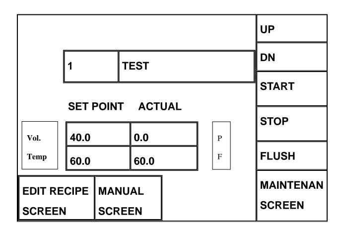
To use a preset water amount and temperature controls (i.e. a recipe), or to add another recipe, tap the "RECIPE SCREEN" button from the manual screen. Use "UP" and "DN" buttons to navigate up or down the recipe list. Tap the desired recipe to use the presets in the recipe. To add or edit a recipe, tap the "EDIT RECIPE SCREEN". This will take the user to the next display:
