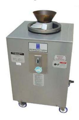
The R900RT Round O Matic Dough Rounder is built with the busy baker in mind. It's Versatility and Simplicity are unmatched in the industry. The R900RT can produce up to 7,200 pieces per hour (depending on size). Dough is automatically rounded into a tight, smooth ball, with no more effort than it takes to drop them into the funnel. No adjustments are necessary when changing the size of the dough pieces. The R900RT is BISSC certified.
