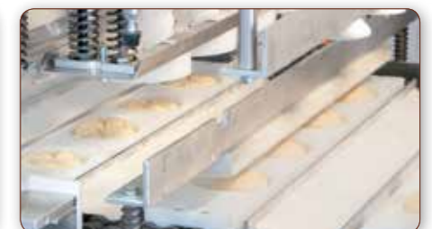
Divider and rounder spreading belts made of plastic (depending on the dough used)
