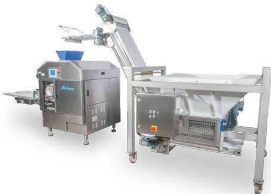
Dough elevating conveyor (up to 200 kg)
