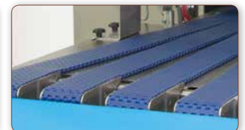
Divider and rounder spreading belts made of plastic (depending on the dough used)
