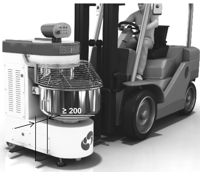
Picture 8 - Machine Lifting up by means of a Fork Lift Truck
